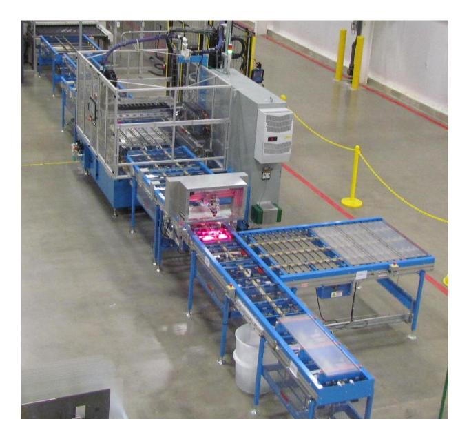
**Automated Edge-Seal Line with Inline bead Inspection**
